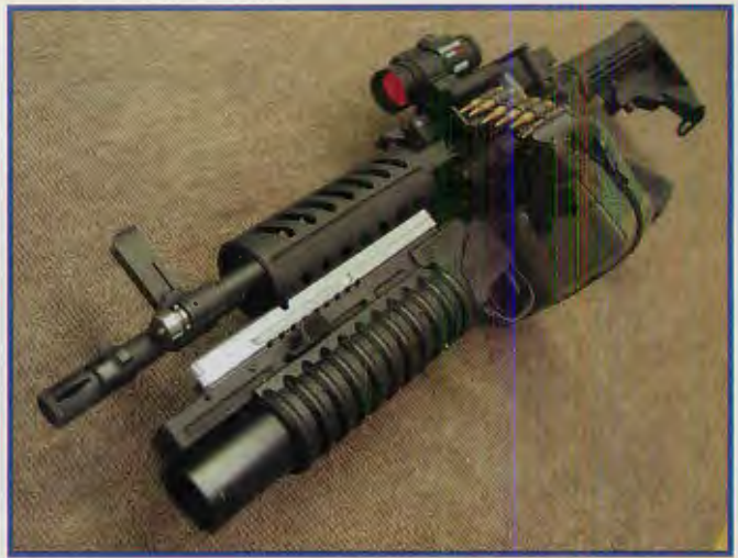
The Shrike 5.56 has been designed to use virtually every accessory, adaptive weapon or sight designed for the M16/M4 weapons systems, including the M203 40mm grenade launcher, shown here with prototype quick-detach mount. Note the Picatinny rail section on QD mount for accepting accessories such as SureFire M900A, when M203 is not employed.
